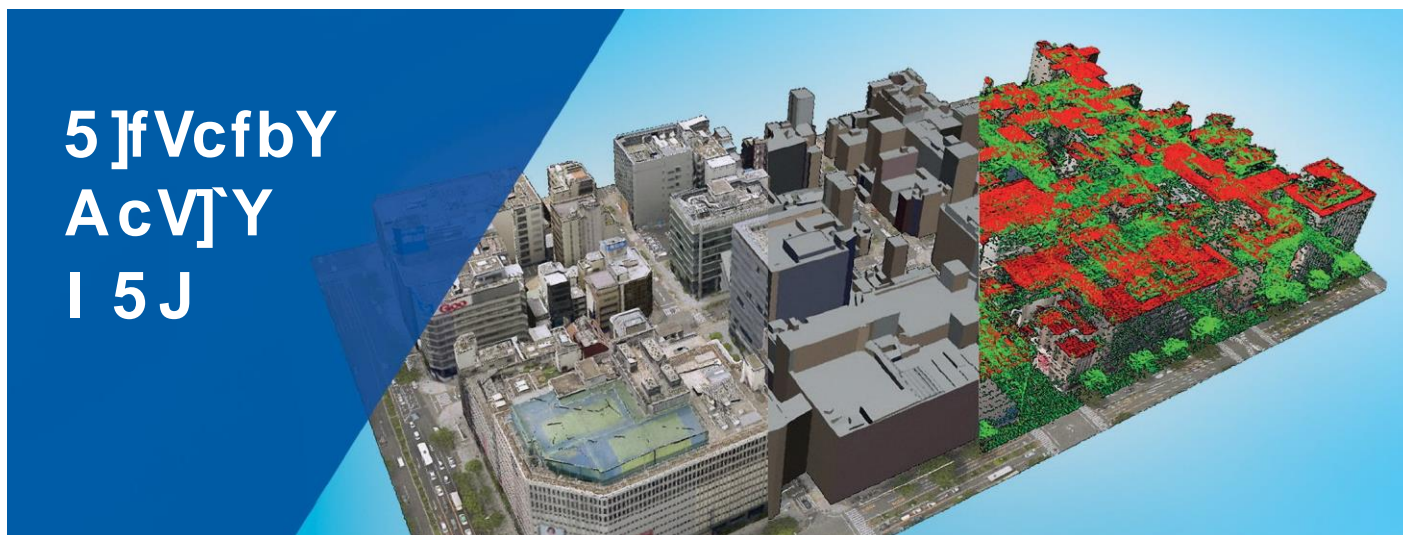
Automatically vectorized and textured 3D city model of Nagoya. Data: Nakanihon Air Service
